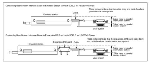
Figure 11 User System Interface Cable Location Example
